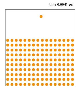
• Example of a molecular dynamics simulation in a simple system: deposition of a single Cu atom on a Cu surface.
